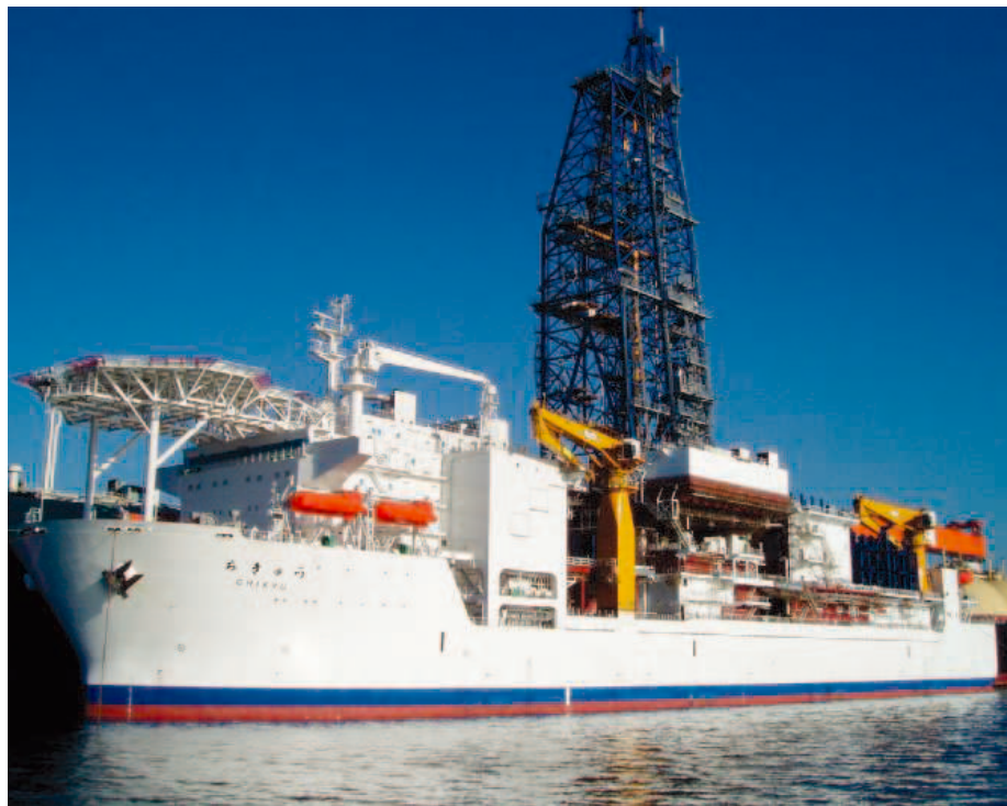
Ocean Goliath. The Chikyu is 45% longer and displaces more than twice the weight of its predecessor in the global ocean drilling program.
